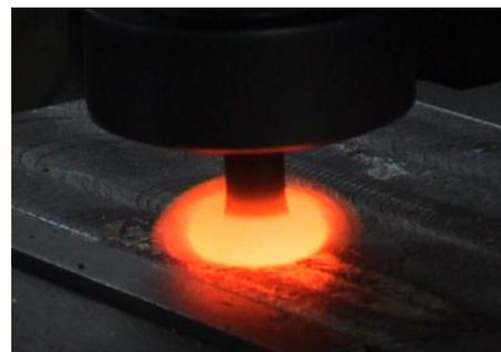
Fig 3.9 a layer of copper coating formed over mild steel
