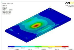
Fig 5.8 Von Mises stress for mild steel
