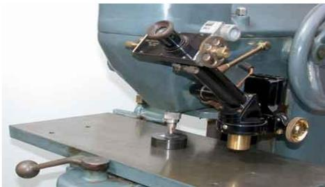
Fig 4.20 Vickers hardness testing machine
