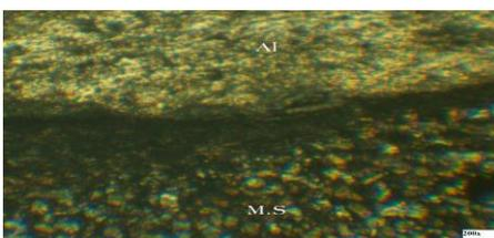
Fig 4.23 the microstructure of the aluminum coating over the mild steel
