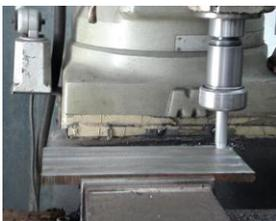
Fig 3.3 Consumable metal rod held in the machine spindle & the M.S plate in the vice
