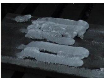
Fig 3.5 after coating of aluminum over mild steel the formation of layers along the plate
