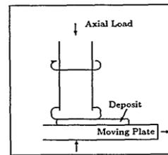
Fig 2.2 Principle mechanism of friction surfacing process
