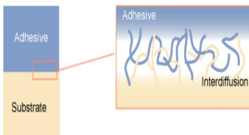
Fig 4.1 Diffusion mechanism
