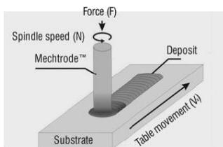
Fig 2.1 the process of friction surfacing is schematically depicted
