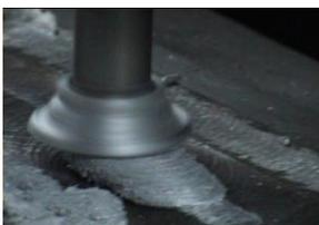
Fig 3.4 Coating of aluminum over the mild steel plate
