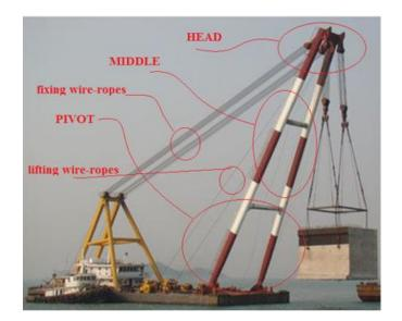
Fig -4: Sheerleg crane, type Welded box girder legs
