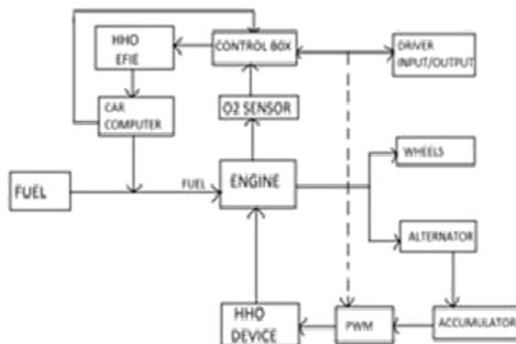
Fig -2: HHO Block Diagram
