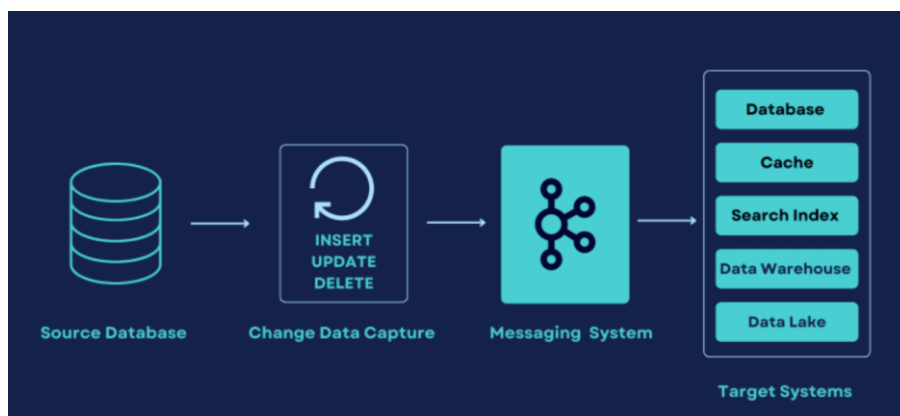
Fig. 4 Working of CDC in conjunction with ETL tools
