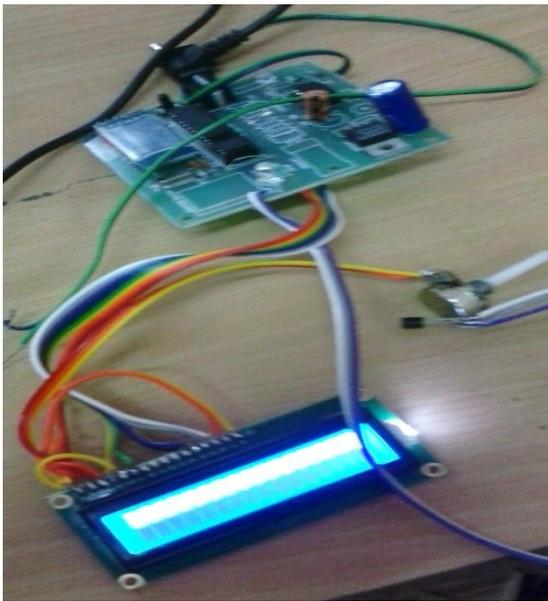
**Fig.4: Temperature measurement in slave module**
