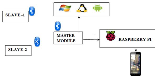
**Fig.1: Block Diagram of Overall System**
