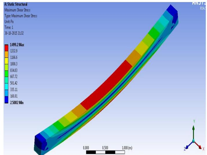
**Fig 3 Shear Stress Of A Beam**
