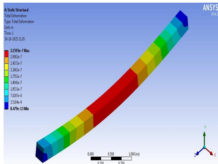
**Fig 4 Total Deformation Of A Beam**
