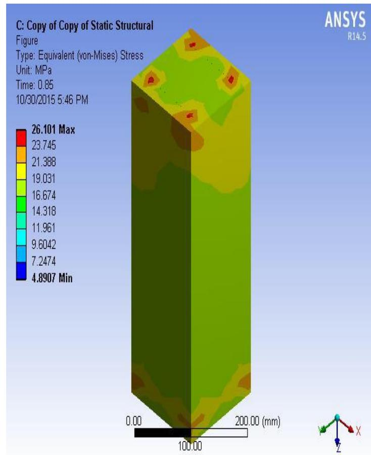
Figure 2.2.4 Von- Mises Stress
