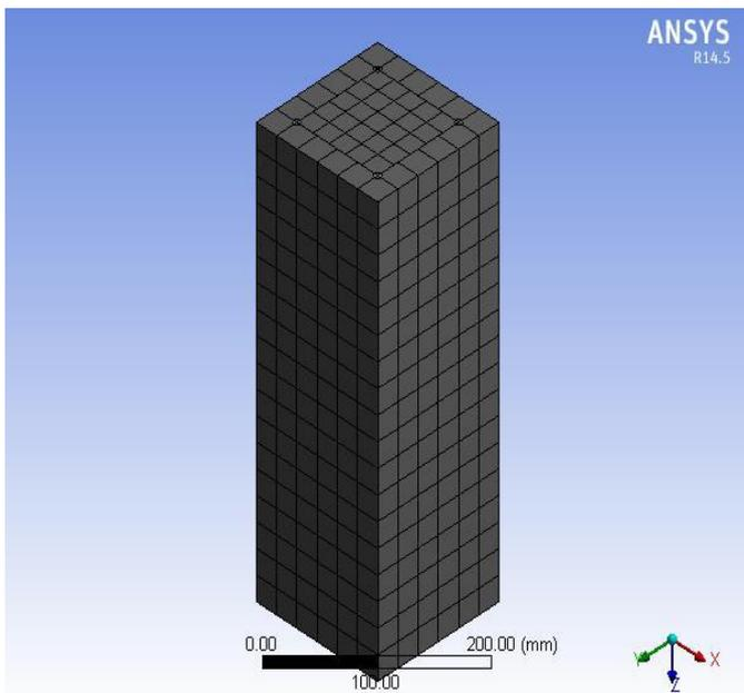
Figure 2.2.2 Design of column using ansys
