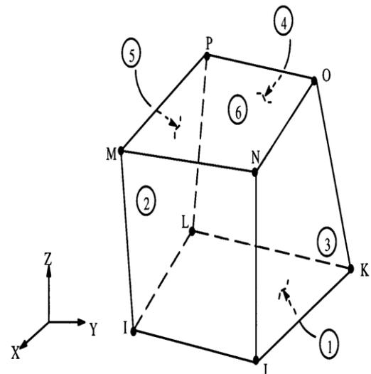
Figure 2.2.1 Solid65 Element Detail
