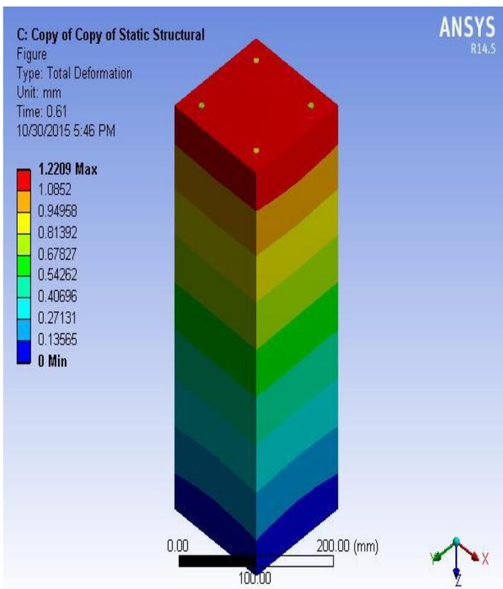
Figure 2.2.3 Deformation of the column
