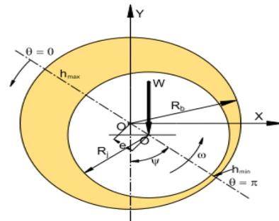
Fig 1: schematic diagram of circular Journal bearing.
