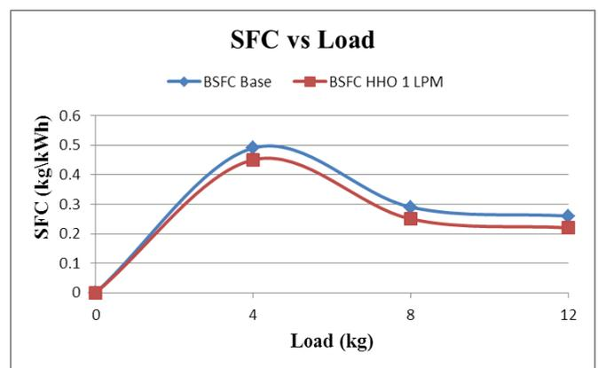
**Figure -3:** Variation of specific fuel consumption with load
