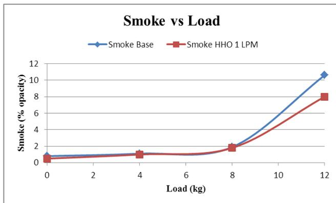
Figure -8: Variation of smoke with load
