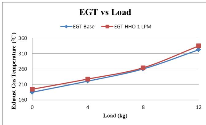
Figure -4: Variation with exhaust gas temperature with load
