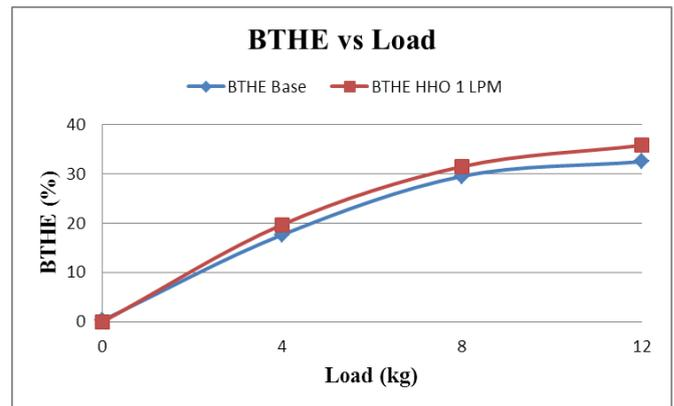
**Figure -2:** Variation of brake thermal efficiency with load
