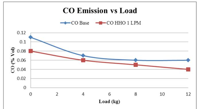
Figure -6: Variation of CO emission with load
