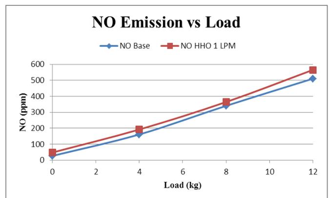
Figure -7: Variation of NO emission with load
