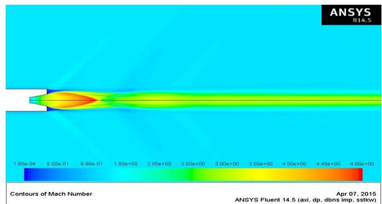
Contour plot of Velocity as Mach number at Mean Sea-level and Jet exit Mach number=4.0
