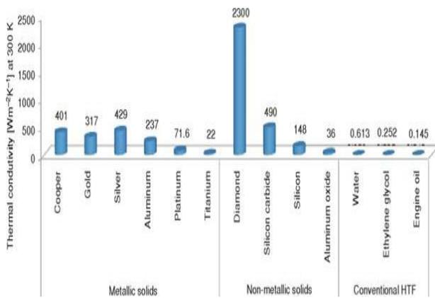
Fig : Thermal conductivity of Metals
