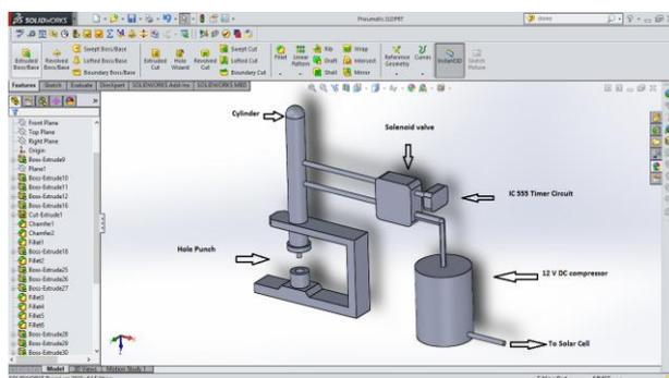
**Fig 3:** Design of Model in SolidWorks
