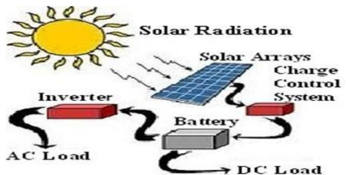
Fig2: Basic Solar Power Generating system
