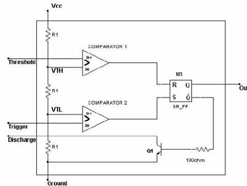
Fig 1 : Block Diagram of IC555 circuit
