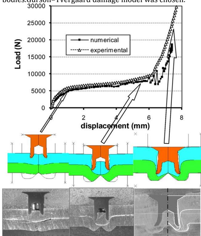
Fig- 4: Deformed shape and load-displacement curve in the 2D FEM model [5]
