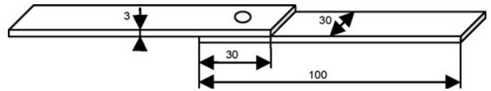
Fig-2: Schematic diagram of the tensile specimen for joint testing.
