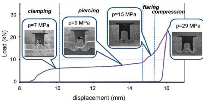
Fig -1: Joining Sequence [5]
