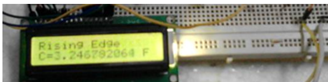
Fig -13: Result indicates the rising edge at conductive electrode with capacitance C value in farad
