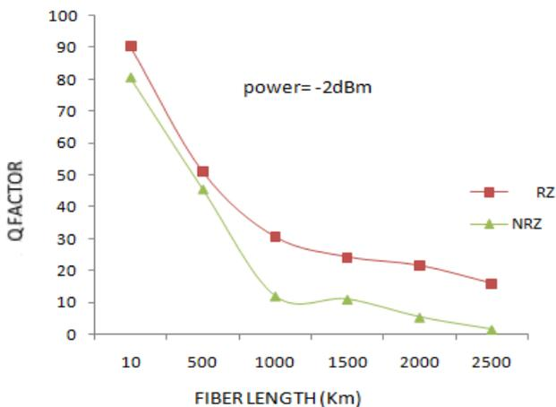
Fig 2 Q factor v/s fiber length (power= -2dBm)
