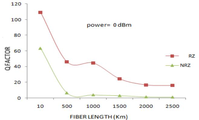
Fig 3 Q factor v/s fiber length (power=0dBm)
