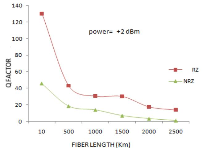
Fig 4 Q factor v/s fiber length (power= 2dBm)
