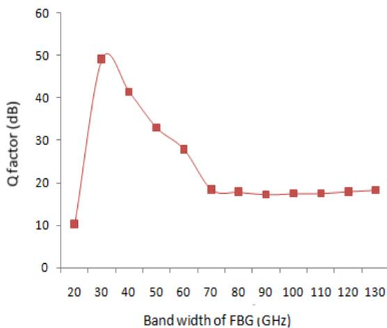
Fig 5 Q factor v/s Bandwidth (GHz)
