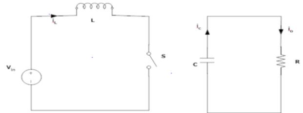
**Fig -2:** ON Mode Circuit
