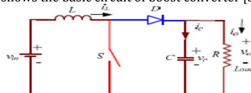
Fig -1: Boost Converter Circuit
