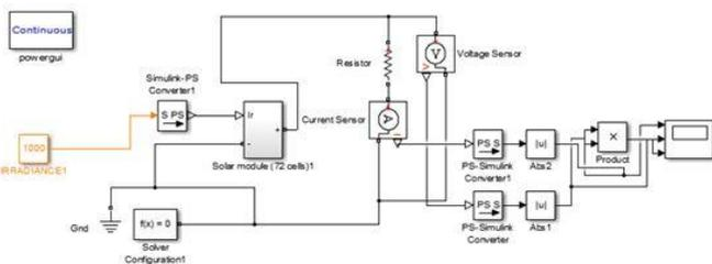
Fig -9: Simulink Model of PV Cell
