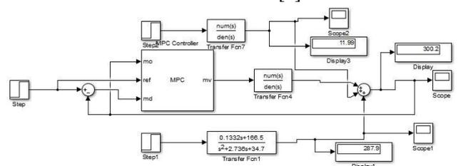
Fig -5: MPC Simulink Model
