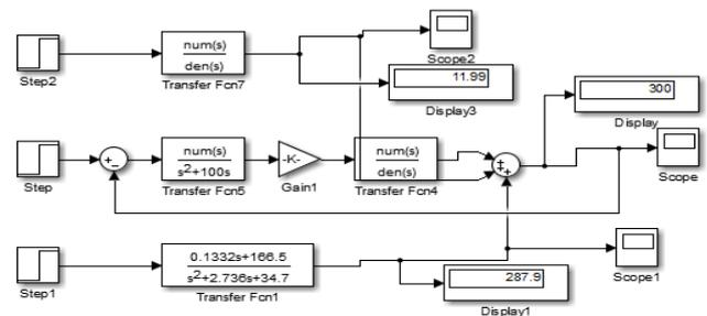
Fig -4: PID Simulink Model
