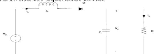
**Fig -3:** OFF Mode Circuit
