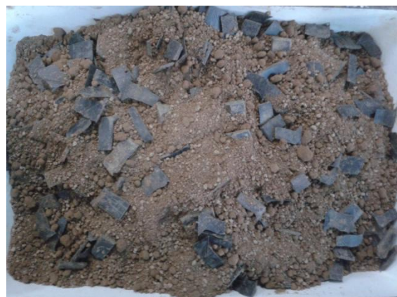
Fig. 2: Soil-Shredded Rubber Tyre Mixture
