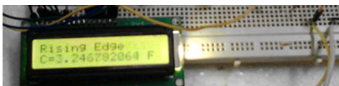
Fig -13: Result indicates the rising edge at conductive electrode with capacitance C value in farad
