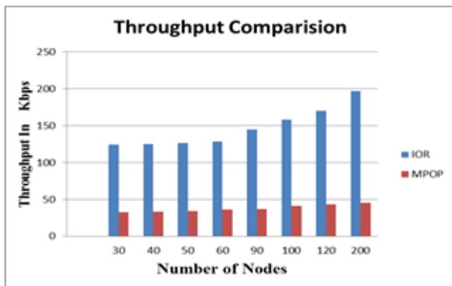
Figure 5.3 Throughput Comparison between IOR and MPOP
