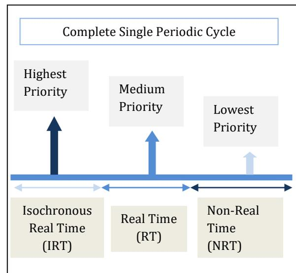
**Fig.2 Structure of PROFINET-IO Single Cycle**
