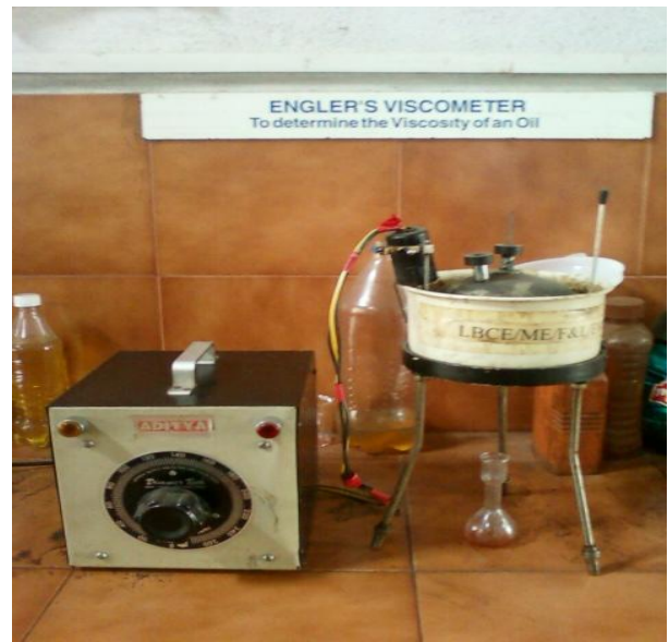
Figure 4.3 Engler's Viscometer and Oil collecting flask
