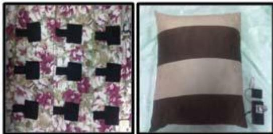
Fig-2: Array of FSR sensor on pillow.
