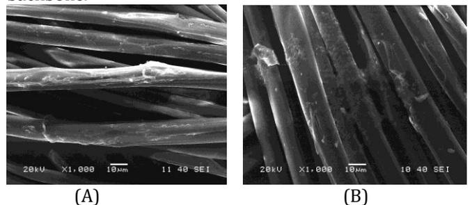
**Figure 6** Scanning electron micrographs of ungrafted silk (A) and AA-grafted-silk (B)
