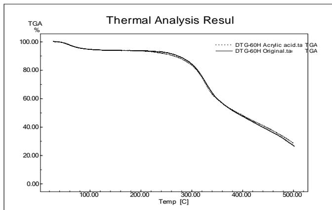
**Figure 7 Thermogram analysis of Original (control) silk and AA-grafted-silk**
