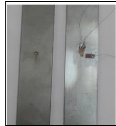
Fig.3.1 MS Plate without strain gauge and Plate with two gauge strain rosette
