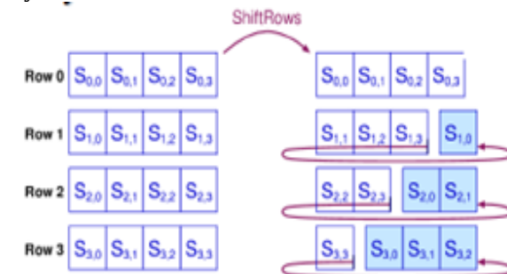
Fig -3: The ShiftRows Transformation
