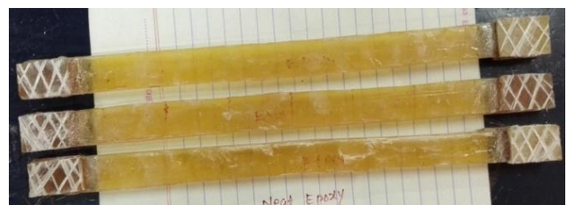
Fig.4 : Tensile Specimen with tabbings at the end
