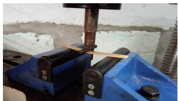
Fig.5 : Specimen loaded for bending test
