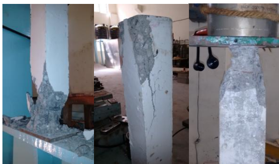
Fig 5: Crack and failure patterns of short columns
