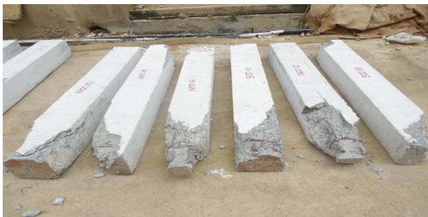
Fig 4: Crack and failure patterns of short columns
