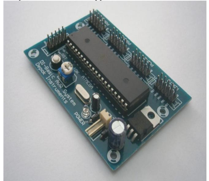
Fig3: AVR (Advance Versatile RISC) Machine.
