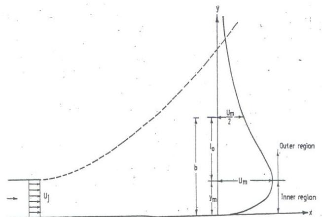
Fig.1 Definition sketch of a wall jet
