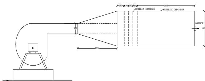
Fig. 3 Schematic experimental set-up
