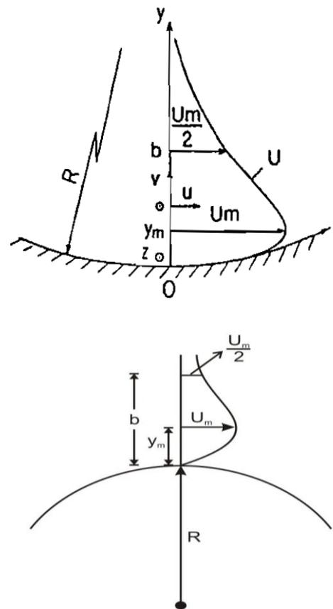
Fig. 2 Definition sketch of curvature parameter  $b/R$
