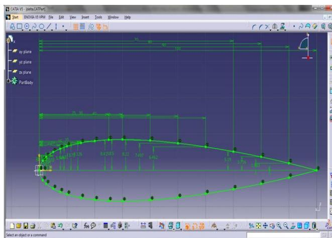
Fig -1: Wing aerofoil design
