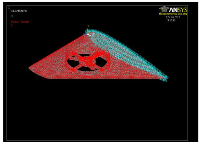
Fig -3: Boundary conditions over rotor wing
