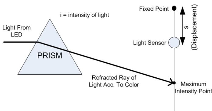
**Fig -2:** Detailed Block Diagram for Maximum Point Detection
