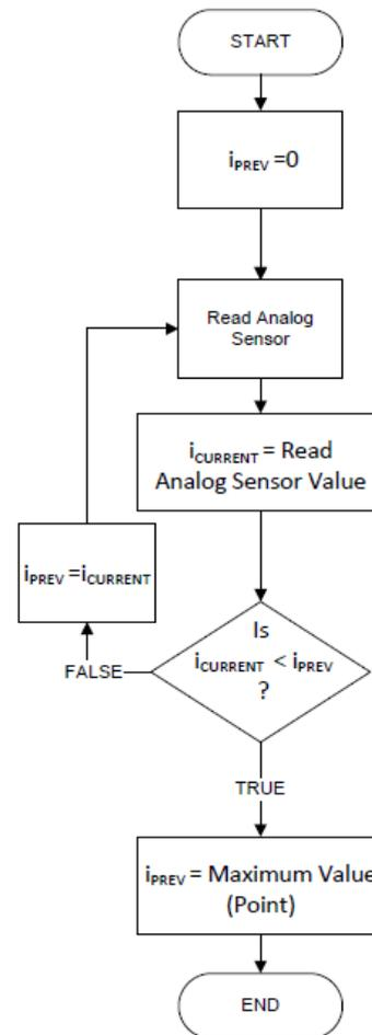
**Fig -3:** Flowchart of Maximum Point Algorithm
