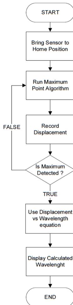
**Fig -4:** Flowchart of Full Working of System
