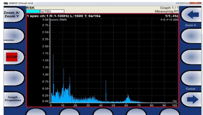
Fig -15: Frequency Response for 26 ft Blade.
