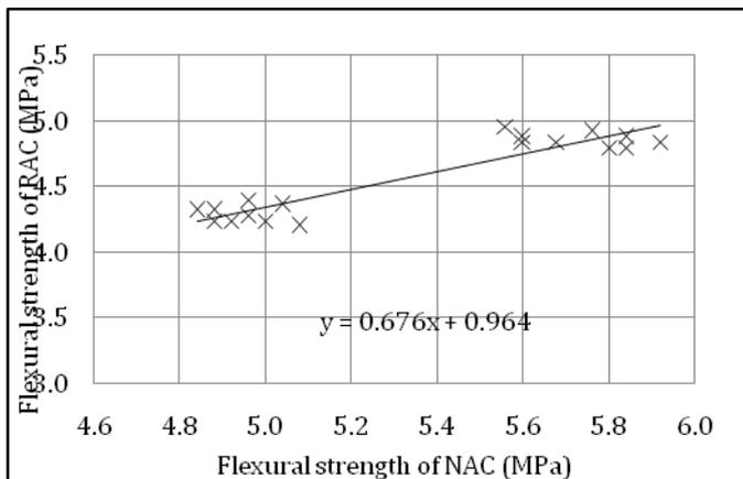
Figure 5: Regression curve to establish the flexural strength of concrete with 50% recycled aggregate.
