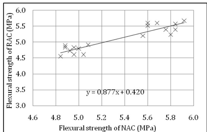
**Figure 2:** Regression curve to establish the flexural strength of concrete with 20% recycled aggregate.
