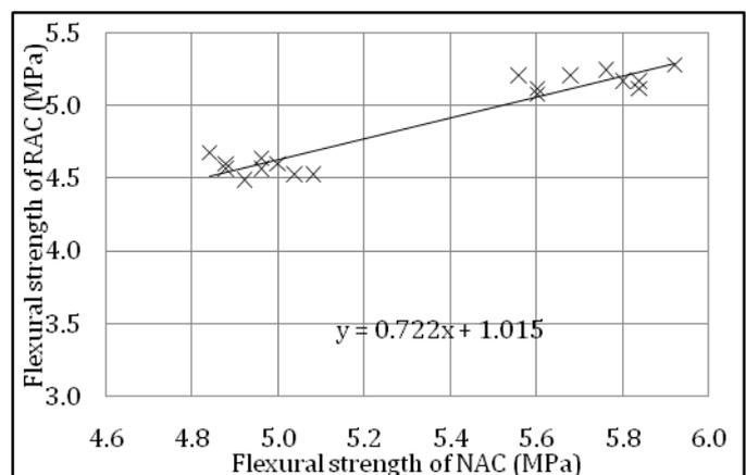
**Figure 3:** Regression curve to establish the flexural strength of concrete with 30% recycled aggregate.
