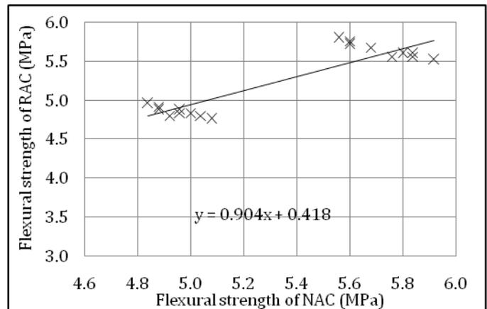
**Figure 1:** Regression curve to establish the flexural strength of concrete with 10% recycled aggregate.
