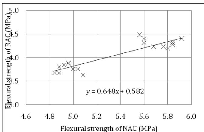
Figure 6: Regression curve to establish the flexural strength of concrete with 80% recycled aggregate.
