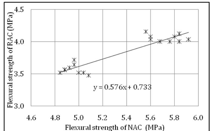
Figure 7: Regression curve to establish the flexural strength of concrete with 100% recycled aggregate.
