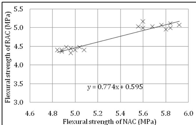
Figure 4: Regression curve to establish the flexural strength of concrete with 40% recycled aggregate.
