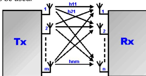
Fig-2 General outline of MIMO system antenna
