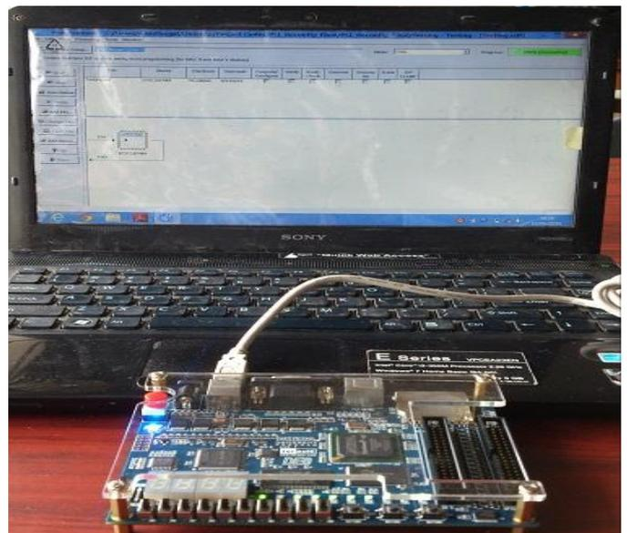
Fig -3: Hardware setup for TRNG.
