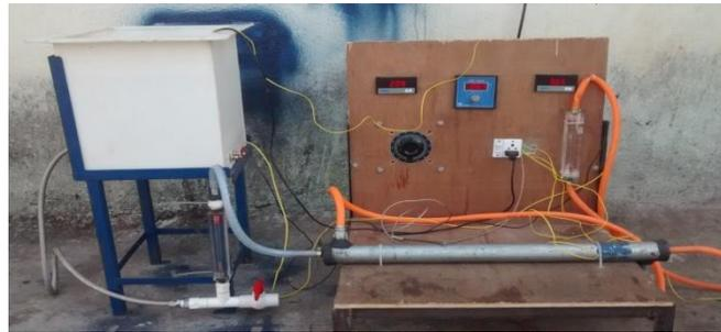
Fig 1 : Experimental set up of double pipe heat exchanger
