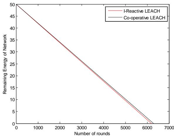
Fig-8 Rate of energy consumption of co-operative LEACH
