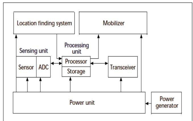
Fig-2 Components of Sensor Node [2]
