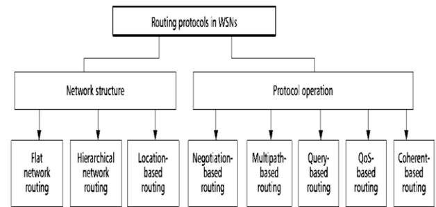
Fig-3 Classification of routing protocols
