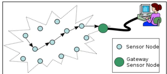
Fig-1 Architecture of Wireless Sensor Network [1]
