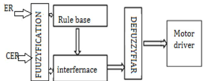
Fig. 2. Block diagram of fuzzy logic controller .
