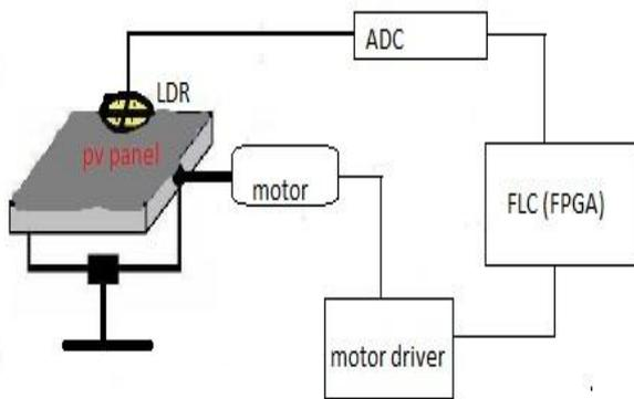
Fig.1 A Block Diagram Of Sun Tracking System
