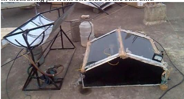
Fig -1: Experimental setup of Double slope with hybrid The photo graph of still with parabolic collector is as shown in the Photo The collector is placed due south at a tilt angle equal to the location. The all other arrangements remain same as single slope with hybrid.
