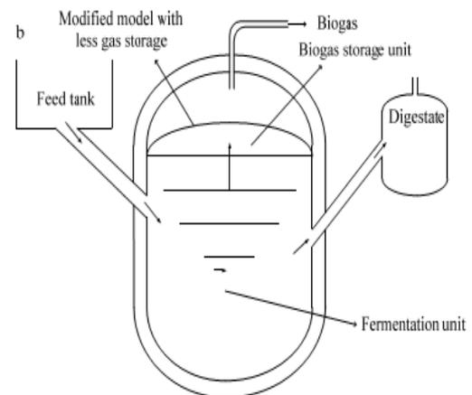
Fig -2: Schematic Diagram of Fixed Dome Digester
