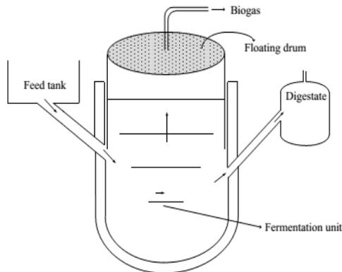
Fig -1: Schematic Diagram of a Floating Drum Digester
