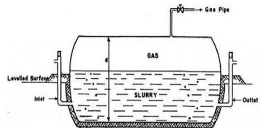
Fig -3: Flexible Bag Type Digester
