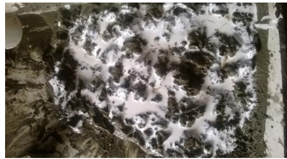
Fig no 1 - polymer and concrete mixture.
