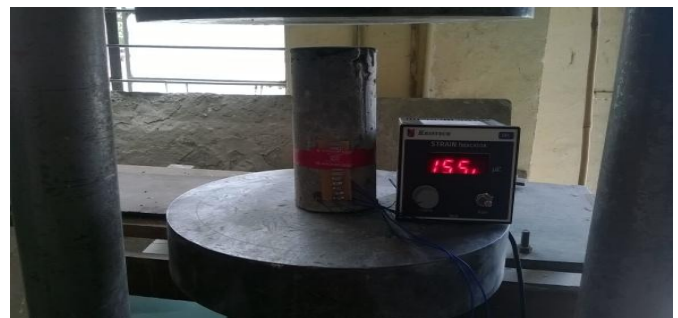
fig no 2- Experiment set up of the with stain indicator
