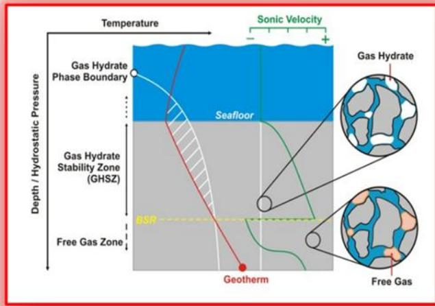
Figure-5: Hydrate stability zone (HSZ) in subsea sediments.
