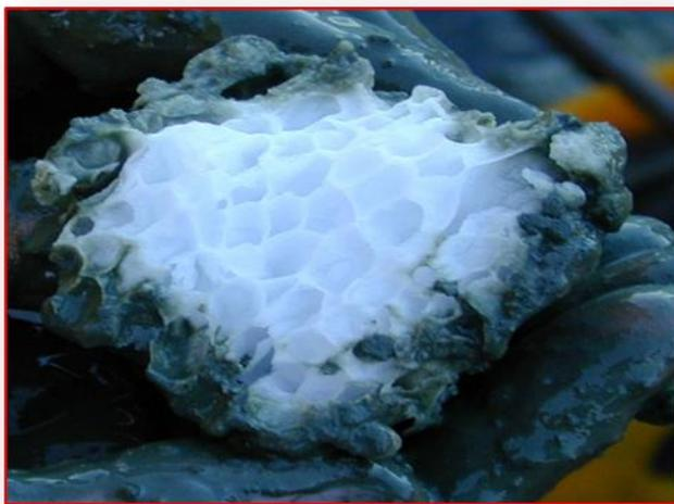
**Figure 4:** Specific structure of a gas hydrate piece
