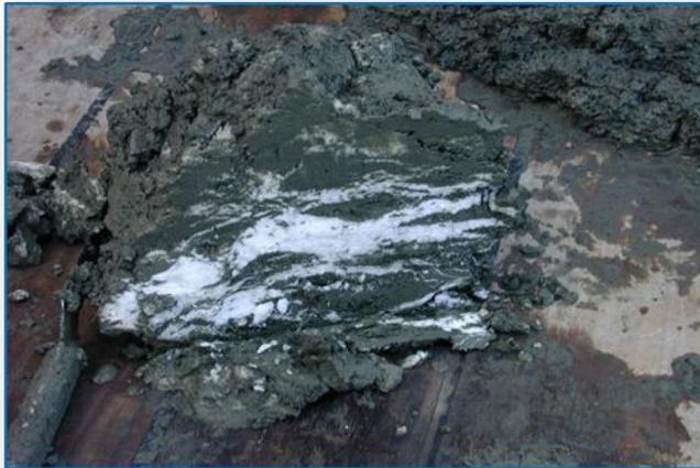
**Figure-3:** Gas hydrate bearing sediment
