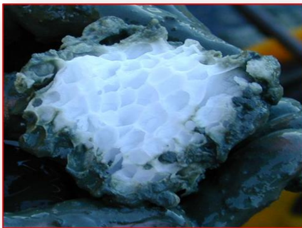
Figure 4: Specific structure of a gas hydrate piece
