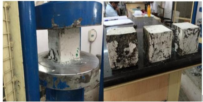
Fig -3Cube specimen under test
