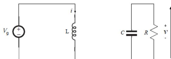
Fig. 8: (a). Buck-boost converter when Q is ON
