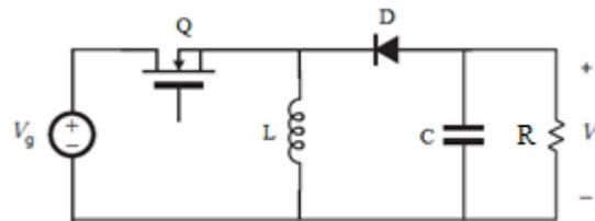
Fig -7: Buck-boost Converter Circuit
