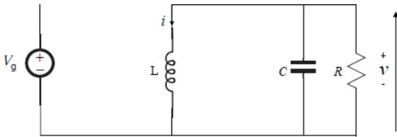
Fig. 8: (b). Buck-boost converter when Q is OFF
