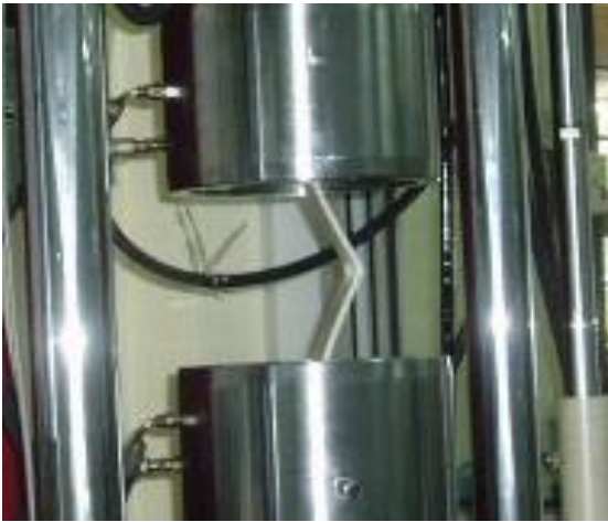
Fig 4 Compression of specimen
