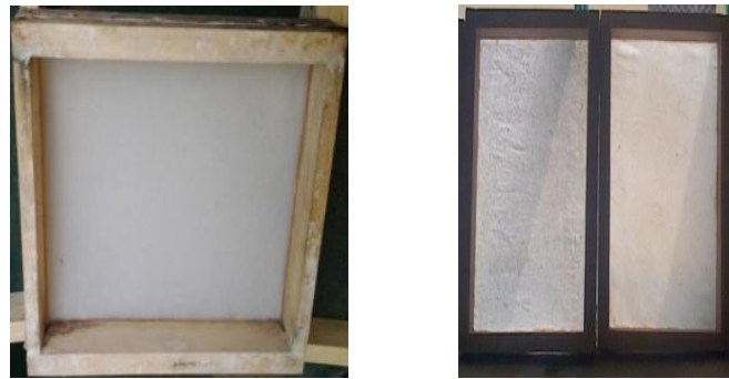
Fig 5: Blended Fibres spread on a paper former and Air-Drying of paper
