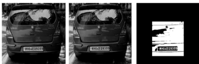
(a) Gray scale (b) Median Filtering (c) Binarized Mask Fig -4: Pre-processing Stages
