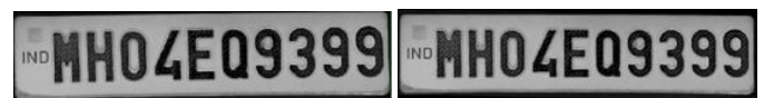
(a) Before Angle Correction (b) After Angle Correction Fig -7: Angle Correction using Radon transform
