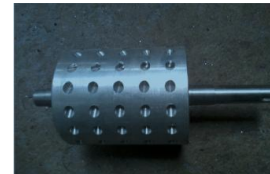
Fig-4: Cavitation heater rotor side view after machining.
