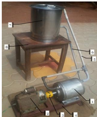
Fig-6: Cavitation heater assembly experimental setup.
