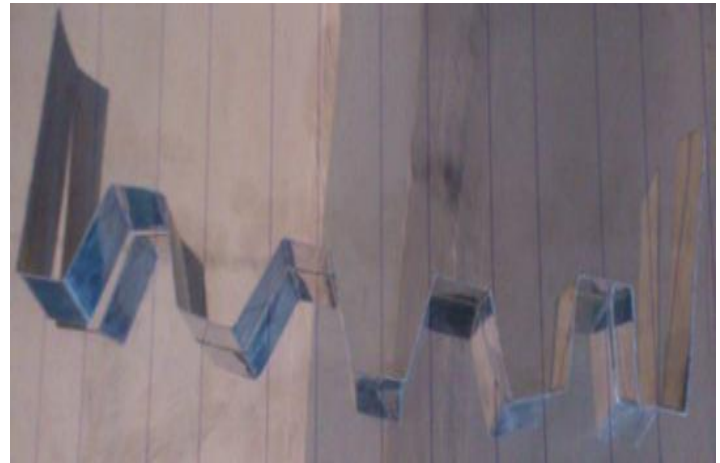
Fig -7: Actual trapezoidal portion of evaporator
