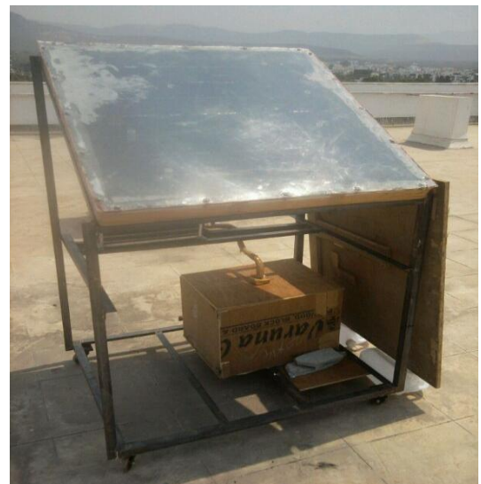
Fig-10: Actual system of ice-maker
