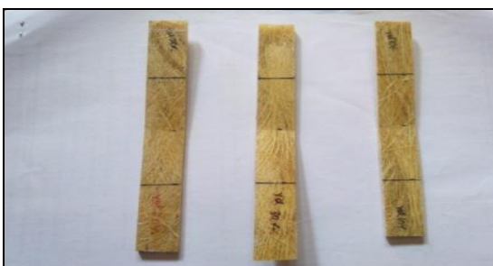
Fig 4.3 Flexural tested specimens
